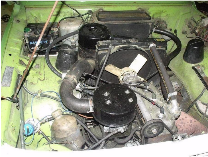
Figure 2: The Wartburg 353, 1.0 two-stroke engine
